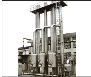
Falling Film Evaporator
